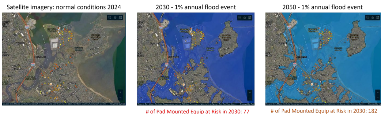
Figure 23: Example from WICT of National Grid’s pad-mounted equipment flood risks in a coastal section of Quincy, MA. In this area, 77 underground pad-mount equipment sites are at risk of a 1% annual probability flood event in 2030 and an additional 105 sites are at risk in 2050, for a total of 182 sites.
