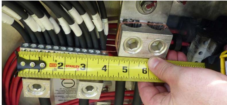
Figure 2-12 Arc initiation in the combiner box for test 27
