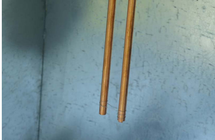
Figure 2-5 Arc initiation wire in place prior to test 1
