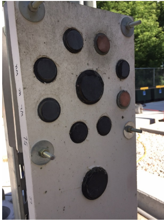
Figure 2-3 Multi-sensor calorimeter array
